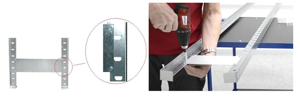
Between the two posts you must attach two spacer plates using M6x10 screw bolts and M6 nuts. One distance plate must be located on the upper side and the other on the lower side. Two posts, two footplates and two spacer plates make up a sideframe.
