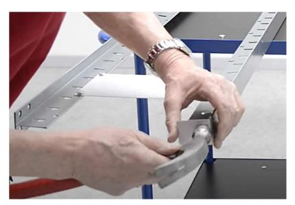
Use a mallet to attach the footplates under the posts. You will need to use a mallet to fix the triangular end between the two sheets of metal. The narrower side of the openings inside the post must be facing the floor.
